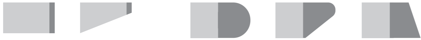
SQUARE 30/38mm thick top CHAMFER 30mm thick top BULLNOSE 38mm thick top CHAMFER DELTA 38mm thick top CLIFF 38mm thick top
